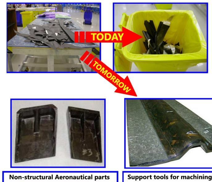
Figure 1 – Possible uses of scraps from machined prepreg material
